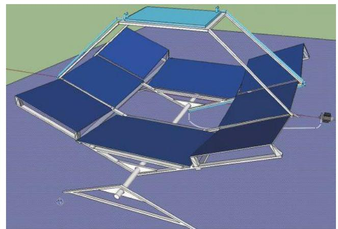
**Eight mirrors focused on a PV solar panel with water cooling.**
